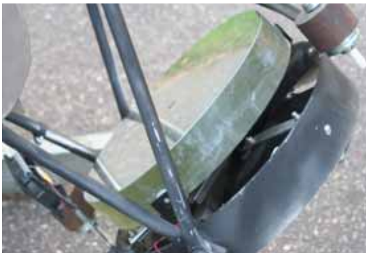
The main 14" mirror inside its open truss support structure
