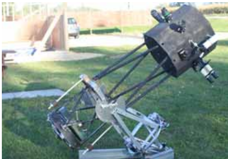
The 14" Newtonian with seven focusers at Cherry Grove Observatory.
