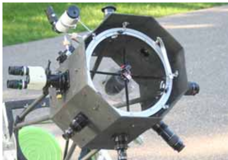
Detail of seven-focuser rotating secondary cage on the 14" Newtonian.
