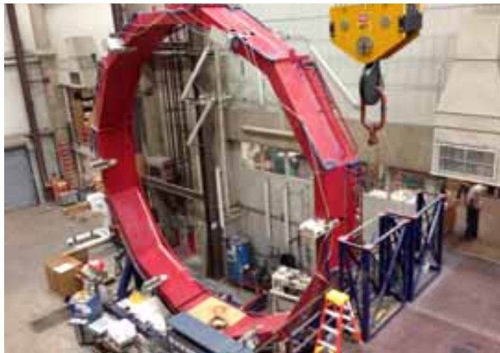
This is an empty frame standing vertically. It will be lowered flat when they are ready to pour glass-making materials
