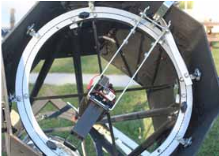
Detail of rotating secondary cage. Inner ring of Lazy Susan is fastened to the truss tube. Outer ring is fastened to the octagonal cage holding the eyepieces.
