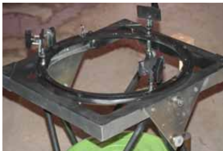
The rotation mechanism for the entire 14" truss tube. This consists of a Lazy Susan attached to a square aluminum frame.
