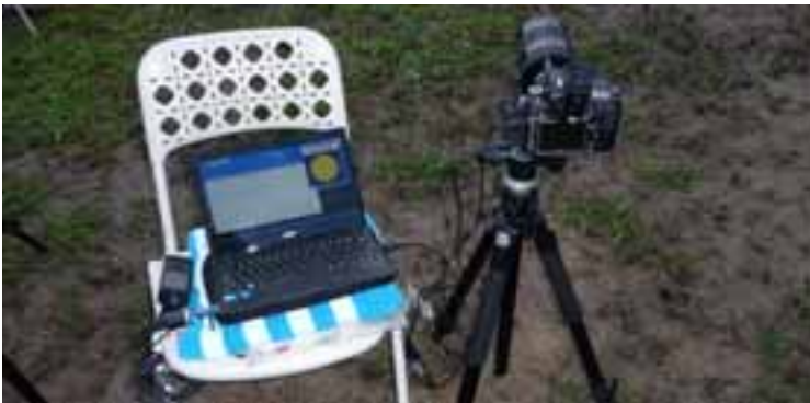
My equipment for the eclipse. I used a Nikon D7000 DSLR with a 1000mm mirror lens controlled by a computer running Eclipse Orchestrator and connected to GPS to ensure accurate timing.
