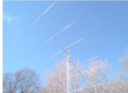
Figure 2: A 6-element force 12 21MHz mono band yagi antenna (44-foot boom) mounted on a 24-foot tower with an alt-azimuth computer-controlled tracking system to track the Sun or Jupiter at W3FAF RO.
