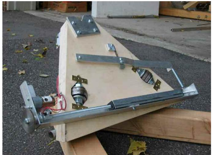
*This shows the base for the 20-inch, including the bearings and the motor drive system.*
