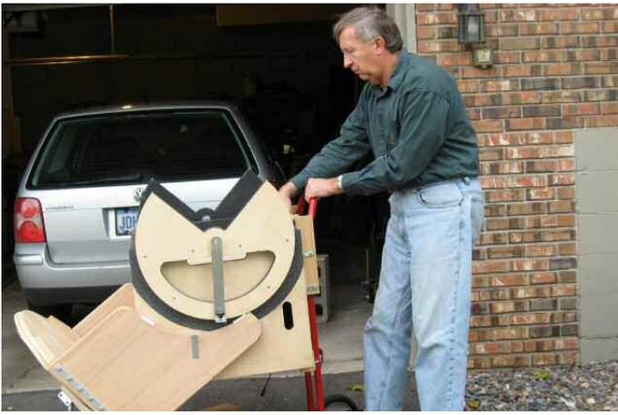
*This shows how I load the 105-pound mirror box onto the fork with the help of the 2-wheel hand truck that I modified for this purpose.*
