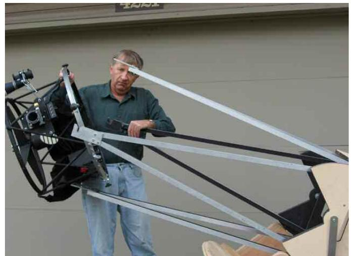
*This shows how I attach the secondary cage without needing to climb a ladder.*
