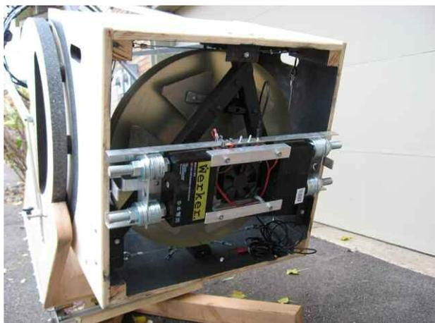
*This is the back of the 20-inch mirror box, also showing the fan/battery/counterweight assembly.*
