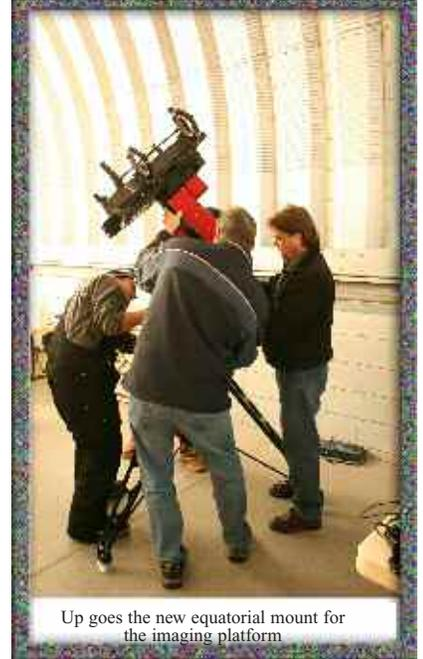
Up goes the new equatorial mount for the imaging platform
