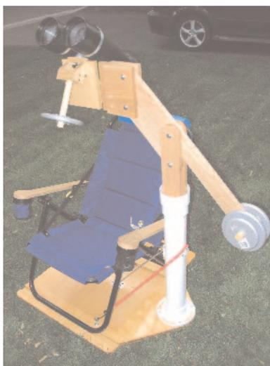
The bino chair consists of a rotating base for a reclining folding chair and a pier for a parallelogram mount. By rotating as a unit you can easily track to any spot in the sky, and the parallelogram mount is counter-weighted to balance the weight of the binocular in any dimension. Also, with a parallelogram mount, you can position the binos virtually anywhere and you can also swing them out of the way to get in or out of the chair without contortions.
