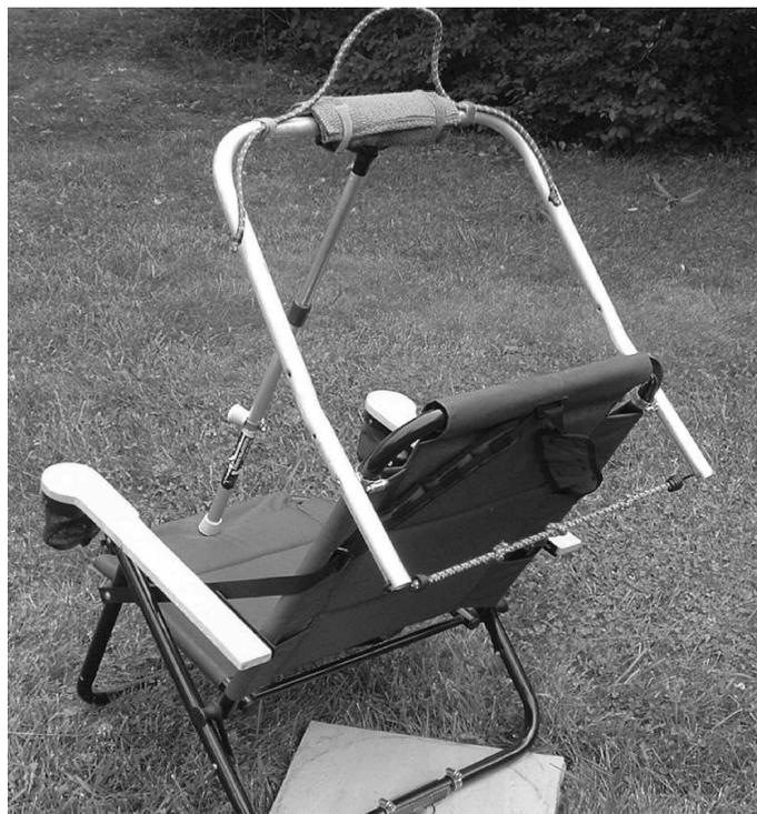
Finished chair, showing U-assembly mounted on pivots, with telescoping snow brush handle, binocular support pad, and bino-support bungee. See also azimuth pivot and baseplate at back leg, and bungee cord across ends of U.
