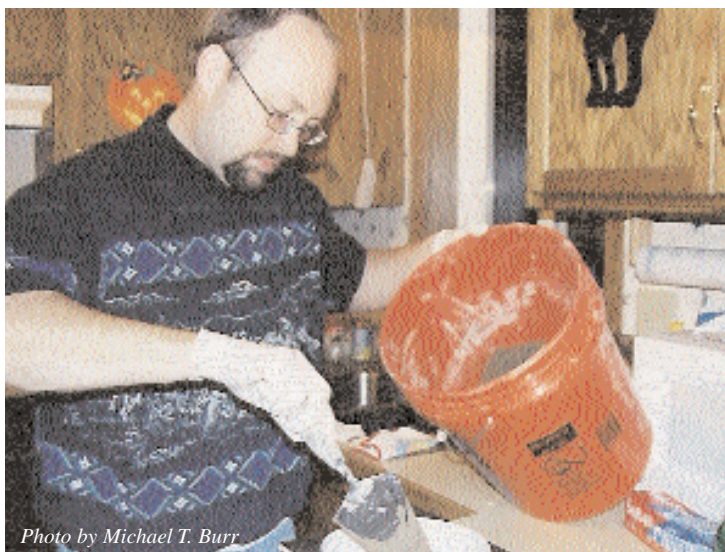
Photo by Michael T. Burr One of the many fun parts of ATMing is making tile tools for grinding mirrors. Almost any plaster or concrete-like substance will work for a tool foundation. Here the author is using cement to cast a sub-diameter foundation for grinding a pair of 10" mirrors.)
